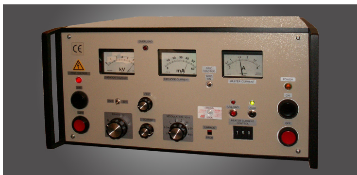
VR6-MU power supply for operating QS1 BWO's
