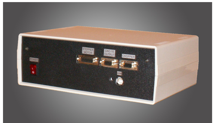
Data Acquisition Unit (DAU) for controlling BWO spectrometer systems.
