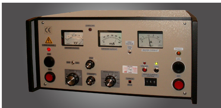
VR6-MU power supply for operating QS1 BWO's
